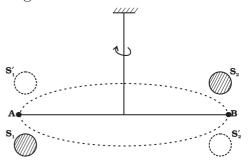
Fig. 7.6 Schematic drawing of Cavendish's experiment.  $S_1$  and  $S_2$  are large spheres which are kept on either side (shown shades) of the masses at A and B. When the big spheres are taken to the other side of the masses (shown by dotted circles), the bar AB rotates a little since the torque reverses direction. The angle of rotation can be measured experimentally.
