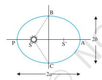
**Fig. 7.1(a)** An ellipse traced out by a planet around the sun. The closest point is P and the farthest point is A, P is called the perihelion and A the aphelion. The semimajor axis is half the distance AP.
