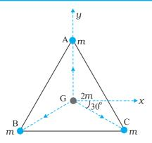
Fig. 7.5 Three equal masses are placed at the three vertices of the  $\triangle$  ABC. A mass 2m is placed at the centroid G.
