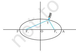
**Fig. 7.1(b)** Drawing an ellipse. A string has its ends fixed at  $F_1$  and  $F_2$ . The tip of a pencil holds the string taut and is moved around.
